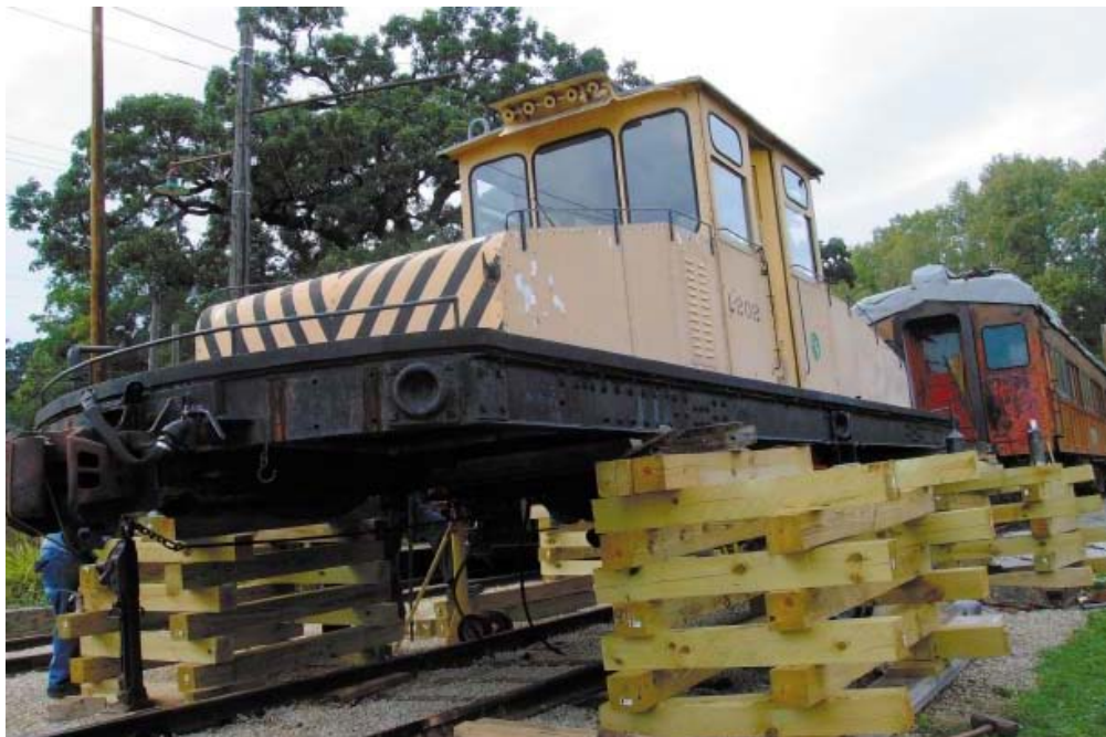
The hole left by the removal of L202's south truck. Don MacBean
