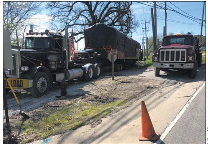
The highway tractor is being hooked up to the dolly to pull the car forward while the tilt-bed recovery truck stands by.
