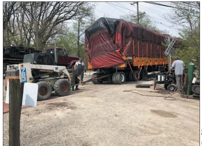
Here the Bobcat is positioning the road dolly or "jeep" under the south bolster of 7.
