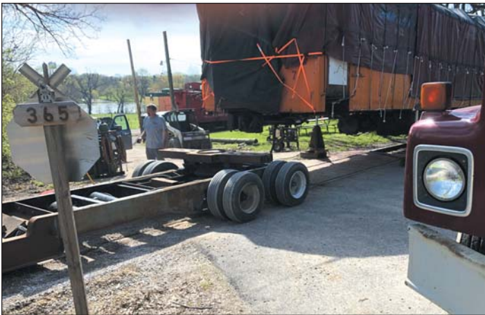
It is moving day for car 7 with the north end receiving its highway dolly in place of its truck.
