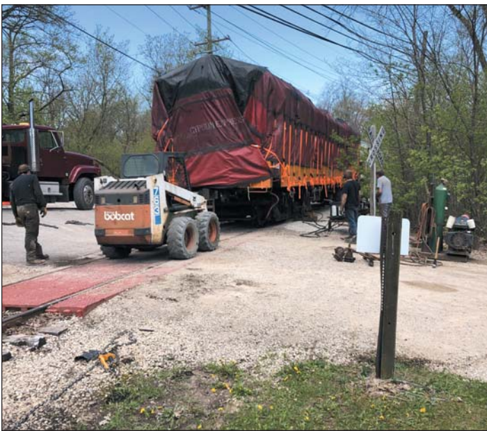
The mover's Bobcat is in place while the jacks are set up to lift the south end of the car.
