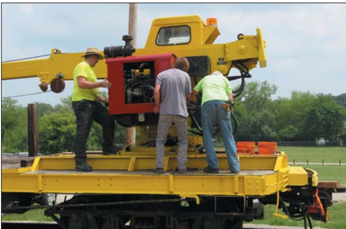
It takes three to install the engine shroud with Jeff Bennett, Chris Nelson and Mike Gilles doing the honors on June 28 th .
