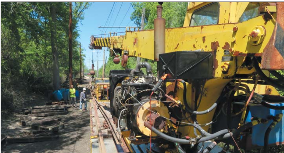
Setting down that second rail on the deck S-314 on May 31 st . Locomotive 5 towed the crane which is on a Skokie Shop made flat car constructed from an old streetcar frame.
